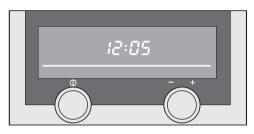
The **On/Off switch** on the left can only be pressed. It does not rotate. Pressing it lightly switches the steam oven on or off. A stronger press will release the switch or push it back in again.
